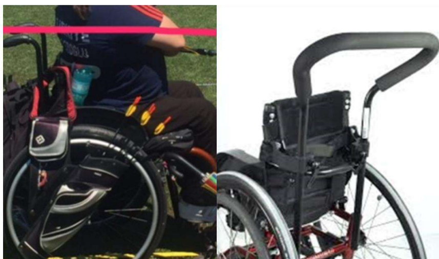
Image 3: Push Handles Not Attached to Wheelchair Back
